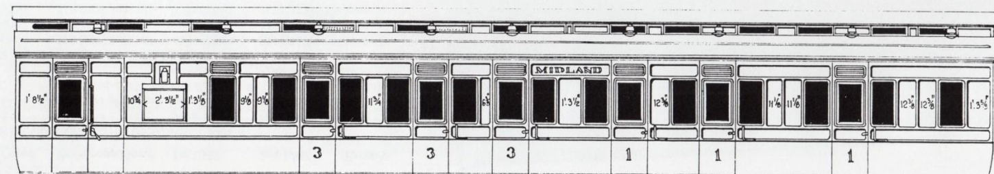
54ft. bogie corridor composite brake
