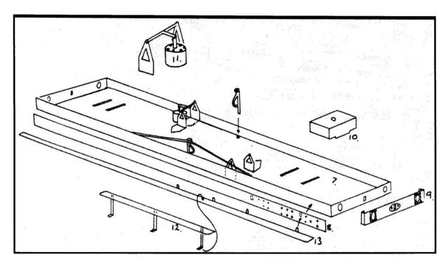
A cast buffer beam is included in this kit, if you wish to use this then remove the etched buffer beam from the floor unit. The choice is left to the builder.
